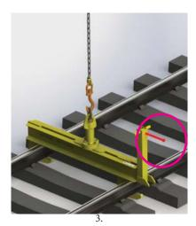
Pull on the beam handles to slide the hooks under the rails
