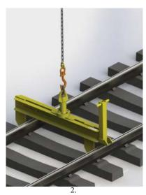
Lower the Panel Lifting Hook Beam until it is resting on the rail heads
